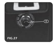
If the machine stops due to overwork or jamming you will need to depress the reset button (1) to be able to resume machine function. Fig. 27.
