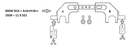
For BMW N12 engines assemble the camshaft locking components as shown.
