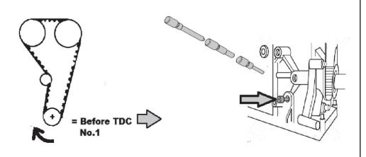
Component 7 = Camshaft Alignment Strap Component 7 is used to lock both the camshafts in their timed position independently of the camshaft pulleys. (for 1.6 Ecoboost Sigma engines use Component 1) Component 9 = Tensioner pin
