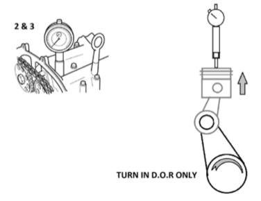
1,2 & 1,4 engines only, use pin 7 to lock the crankshaft in its times position.
