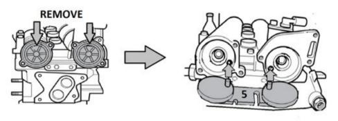
On supercharged models use pins 6 in place of mounting bolts (A) to help guide the charger down and back up again.
