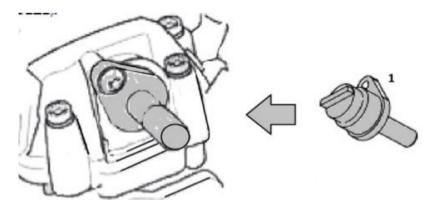
Warning: do not use 1 as a holding tool when loosening or tightening the camshaft sprocket.
