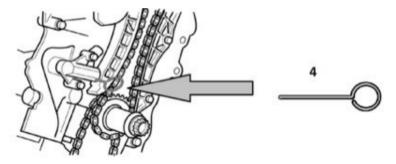
For 1,2 engines only lock the camshaft in position with tool 1.
