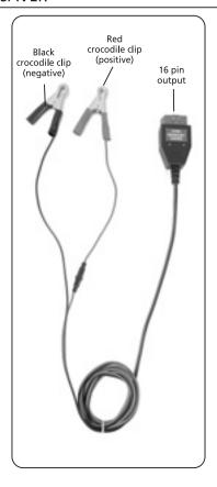
Disconnect the EOBD memory saver from the vehicle. Finally disconnect the EOBD memory saver from its power supply.
