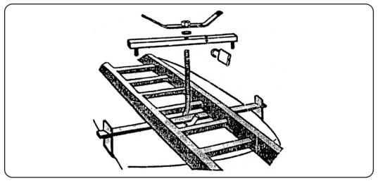
Assemble components as shown above to make two rack clamps (padlock not included).
