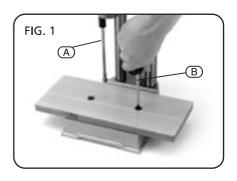
Fix down hold post © to fence D by tightening grub screw with hex. key provided. (Ensure the flat surface of the hold down post in facing the screw).
