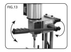
It is important to set the depth stop on the main column this will prevent morticing too deep and possibly damaging the work table.
