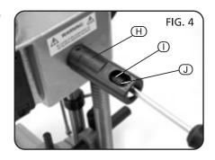
Remove the nut, 2 x washers and spring from the end pf the plunge lever. Fit the lever through the dog chuck and reassemble the washers, spring and nut.
