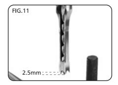
The chisel must be fitted ⑤ so that the open side is to the left or right. The workpiece must travel in the direction away from the open face.
