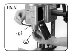
Insert the drill bit and chisel into the hole.
