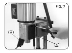
Select the correct reducing bush for the diameter chisel you are using ①. The hole in the bush must line up with the hex. bolt ①.
