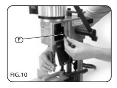
**NOTE:** It is important the bottom point of the bit protrudes 2.5mm below the bottom edge of the chisel (Fig.11).
