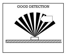
The best detection is obtained by approaching the field of detection at  $90^{\circ}$  to the direction in which the detector unit is facing.
