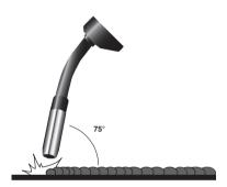
The position of the welding torch is important to achieve a good quality bead. Position the torch at approximately 35 vertically and 75 horizontally and up to 20mm\* distance from the join, 20mm is the maximum that can be achieved on the maximum setting. Ensure the gas shroud remains clean of spatter as a build up will start to reduce the flow/effects of the shield gas. Likewise and more importantly the wire feed tip must be kept clean to avoid the wire becoming blocked or restricted.
