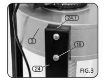
Pass the two (M8 x 45mm) bolts (33) through the handle (8), the upright (24), the spacing block (24.1) and the collection bag ducting (4) and secure in place with the (M8) nuts (12).
