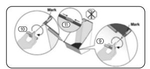
7. Attach the hopper crossbar (6) to the handle and assembled hopper ensuring the hopper rods and the handle click securely into place with the clips on the hopper crossbar (6).
