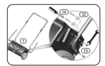
3. Attach left and right supports legs (3) & (4) to the sweeper body (1) and secure using 8mm x <sup>3</sup>/<sub>4</sub>in screws (15).
