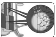
10. Clip the assembled hopper into position on the handle and slot the connectors into the recesses on the sweeper body (1).
