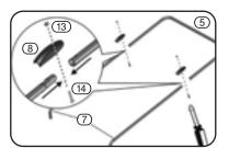
Attach assembled handle section to the sweeper body
