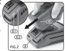
5°C and 30°C. The battery needs to be warmed-up or cooled down in order to prevent damage to the batteries internal components,
