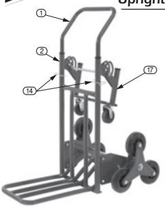
Remove the 2 cotter pins (14) and remove the tubular handle section (1), then re-insert it into the corresponding sockets of the folding rear castor wheel section (17). Align the holes in the frames of both sections and insert the 2 cotter pins (14) to lock in place.
