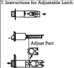
The cam is pushed fully to the right for 70mm backset. (During the adjustment keep two teeth of the cam in the forward position.)
