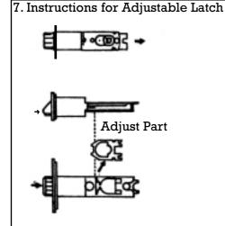
The cam is pushed fully to the right for 70mm backset. (During the adjustment always keep two teeth of the cam in the forward position).
