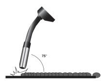
The position of the welding torch is important to achieve a good quality bead. Position the torch at approximately 35 vertically and 75 horizontally and up to 20mm\* distance from the join. 20mm is the maximum that can be achieved on the maximum setting. Ensure the gas shroud remains clean of spatter as a build up will start to reduce the flow/effects of the shield gas. Likewise and more importantly the wire feed tip must be kept clean to avoid the wire becoming blocked or restricted.
