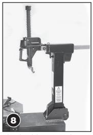
Tilt pneumatic column backwards and hold in place while you insert head and then secure the compression spring with cap and hex. head screw.
