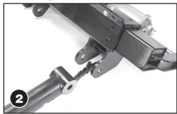
Attach the top arm with control switch.
